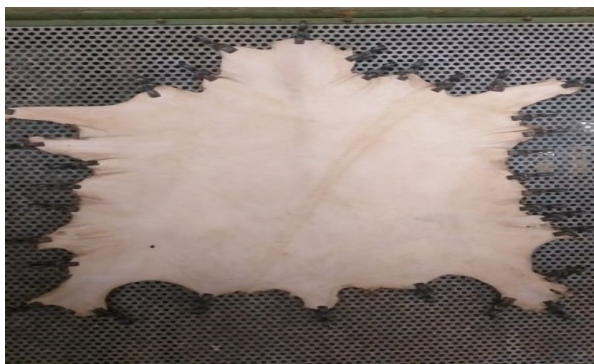
Fig. 3. Representative finished leather insole prepared from extract-enriched vegetable-tanned leather
